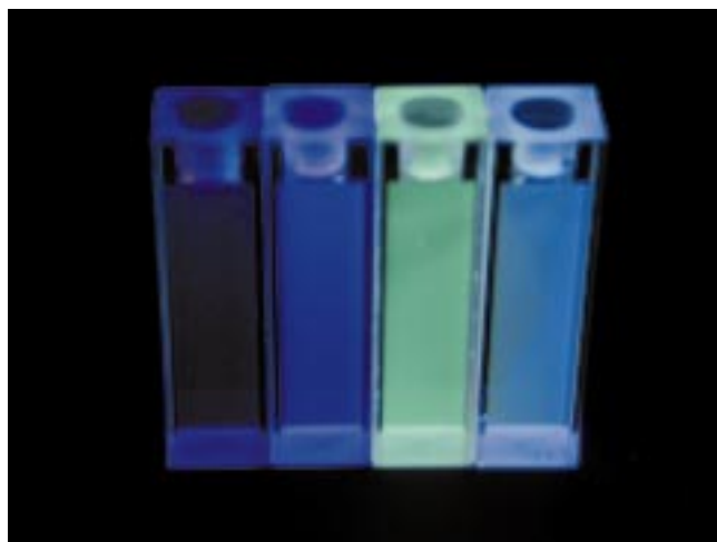
Figure 3. Visible emission observed from samples of 4 and various alkali metal and alkaline earth cations. Left to right: no metal, 4 ·Li + , 4 ·Mg 2+ , and 4 ·Ca 2+ .
